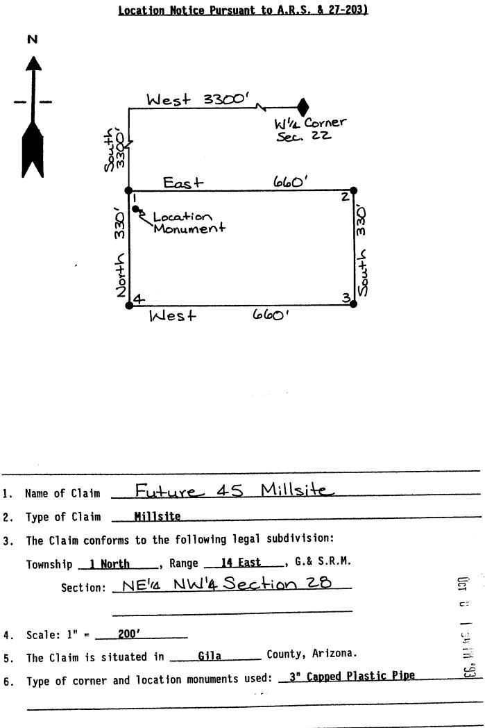
PLAT OF MILL SITE CLAIM (To be Attached to Recorded Copy of
